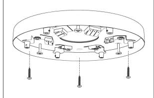
Fixate the mounting plate to the ceiling with screws.
