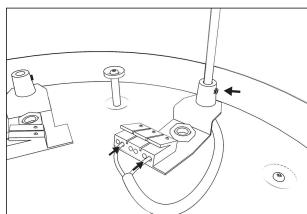
Lead the cables through the cable relief and fixate the cable by turning the screw clockwise.
