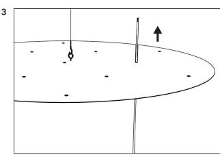
Lead the cables through the cover plate.
