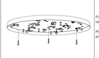
Fixate the mounting plate to the ceiling with screws.
