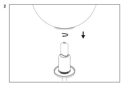
Take the glass globe and carefully place it over the light bulb. Fixate it by turning the glass globe clockwise.
