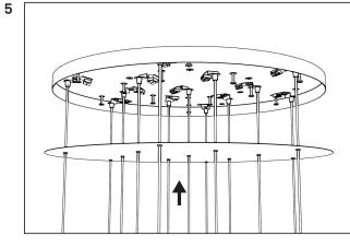
Lead the power cable into the ceiling plate and make sure the cable relief is thightened.
