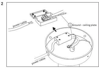
Install the power cable by leading it through either the top or the side of the ceiling plate through the cable relief and into the cable connector. Please make sure the cable relief is tightened.
