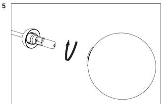
Take the glass globe and carefully place it over the light bulb and socket.
